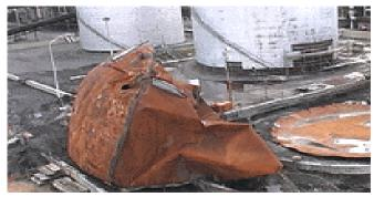
Large sulfuric acid storage tank collapsed after an explosion (Courtesy CSB (11)).
